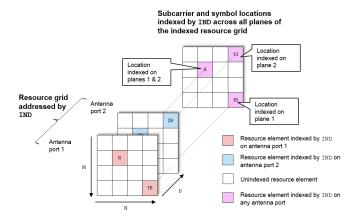
Resource elements are extracted from grid at the symbol and subcarrier locations. The following diagrams illustrate the resource element extraction from a 3D received grid, grid, with NRxAnts = 3.
