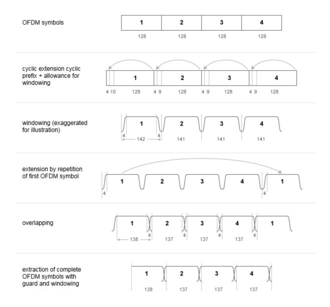
The number of samples used for windowing depends on the number of resource blocks (NRB) and whether the cyclic prefix length is normal or extended. The number of samples is chosen in accordance with the *maximum* values implied by TS 36.101 [1], Tables F.5.3-1 and F.5.4-1.
